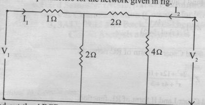
b) Find out the ABCD parameters of the network shown in fig. Also find the image parameters for the network.
